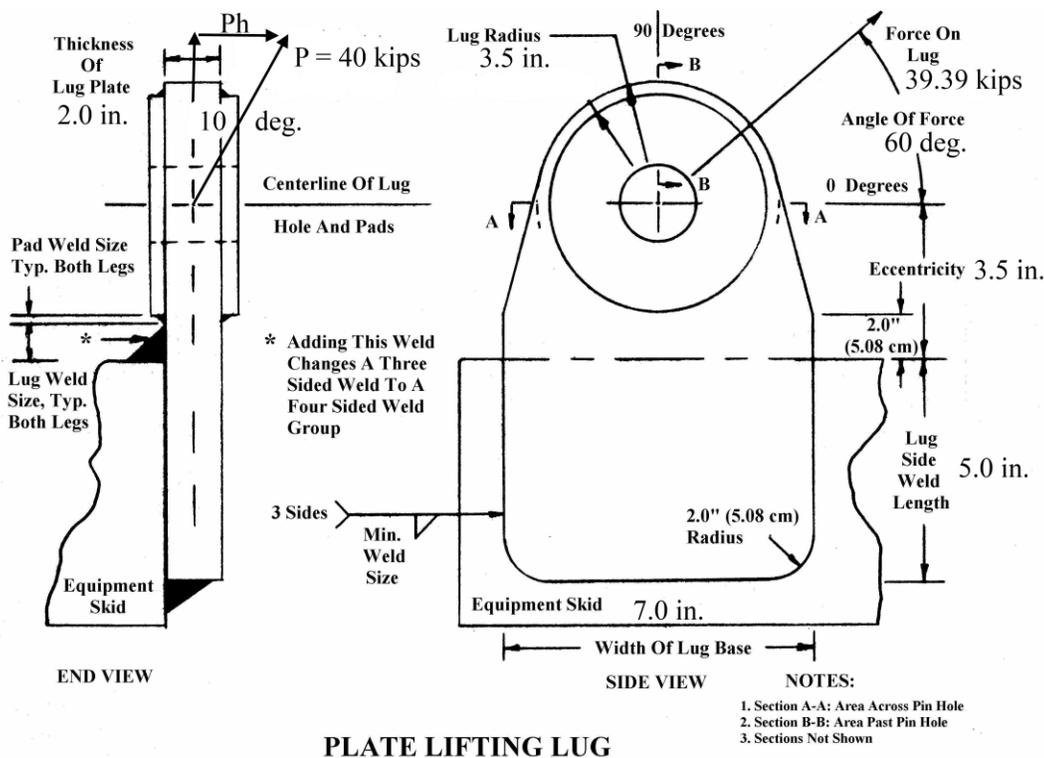
**NOW CALCULATE THE ADDITIONAL STRESS IMPOSED ON THE LUG PLATE DUE TO THE SIDE LOAD:**
